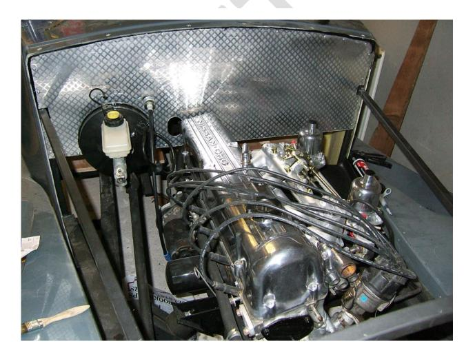
engine is in its original inclined position. In most cases, the standard Datsun gearbox cross-member can be used and simply cut to length if it's too long.
